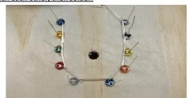
Build Pat's 10 component 14M2 Microcontroller, inserting 10 x pre tinned 100mm coloured wires through the tug holes and solder in pins 0,1,2,3,4,5,c.0,c.1,c.2,c.4 (skip c.3).
