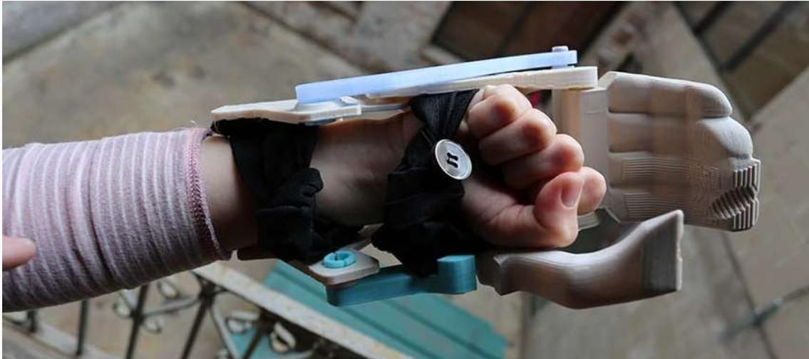
Pictured: Fully 3D printed prosthetic hand by Bold Machines & Field Ready from [3dprint.com](http://3dprint.com)
